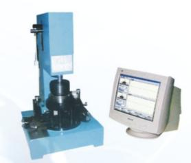
Running Accuracy is an important parameter to assess precision bearing quality. The instrument measuring principle meets ISO standard requirements, it is used to evaluate the quality of finished bearing. The instrument is also applicable to bearing check and acceptance for bearing manufacturers and military users.
