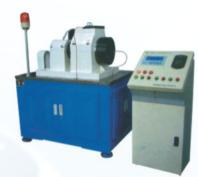
BL series rolling bearing dynamic performance measuring instrument is an mechatronics rolling bearing inspection equipment designed based on National machinery industry standards JB/T7049–93 and JB/T50093–1997. It can detect bearing vibration and temperature and assess bearing life. The instrument has reasonable design, stable performance and will not change the failure mechanism of tested bearings. BL series rolling bearing dynamic performance measuring instrument can be
