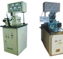
S09 Series Vibration measuring instrument is divided into the bearing vibration measuring instrument and single ball vibration measuring instrument according to the type of measured products.
