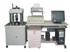
Rigidity is the capability of mechanical components to resist distortion when forceing on it. Its value can be obtained by measuring displacement when the part is impressed by force and become deformed. Now in demestic, there is no specialized measuring instruments for bearing rigidity, most users just calculate bearing rigidity in theory. Some others also use simple
