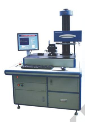
Absorbed the domestic and abroad advance experiences, XM200 surface profile measuring instrument has been improved based on the T2450 roller convexity measuring instrument (ministry of machine-building industry science and technology advancement prize, third grade). It is used to measure surface geometry and macro geometry for many kinds of machine parts.
