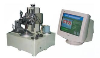
This instrument is designed according to the measuring method regulated in Standard GB307.2-84. It can measure all kinds of bearings bore and outside diameter.
