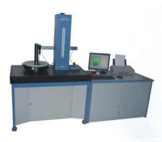
YZD-400 Ultra-precision Cylindricality & Diameter Measuring Instrument can measure roundness,cylindricality,diameter of the machanical components by radial-method,it is widely used in many industries such as aviation,aerospace, automobile,machine,electronic,etc.,it is an indispensable instrument in machining process of the precision components.
