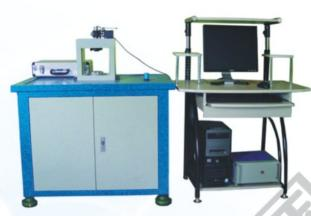
The preload of matched bearing is a key parameter. Its accuracy affects the performance of duplex bearings directly as well as the whole host. When doing the original installation, bearing will have a certain pre-deformation. So the main role of pre-load is that making the bearings skips the initial large deformation stage. It increases the support rigidity significantly. In addition, the matched bearings are used in precision shafting which needs higher accuracy.
